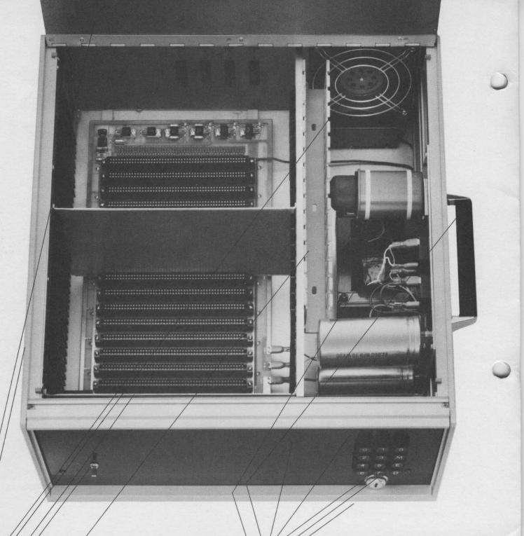
WIRING CHANNEL\*, cord wrap\* and detachable line cord help keep your system neat.
