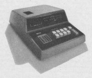
The Altoir VLCT is ideal for machine language programming. It converts a three digit octal code directly into an 8 digit binary code for transmission to the computer and then displays the binary output from the computer in a 3 digital octal format. This allows you to program in octal which is much easier than programming in binary. In addition, the VLCT is much more convenient to work with than using the front panel switches of the Altoir 8800.
