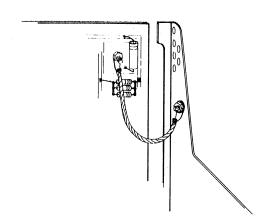
NOTE: At any point where a connection is made to the chassis, first rub the area around the connection point with sandpaper or some other abrasive to remove the anodizing.
