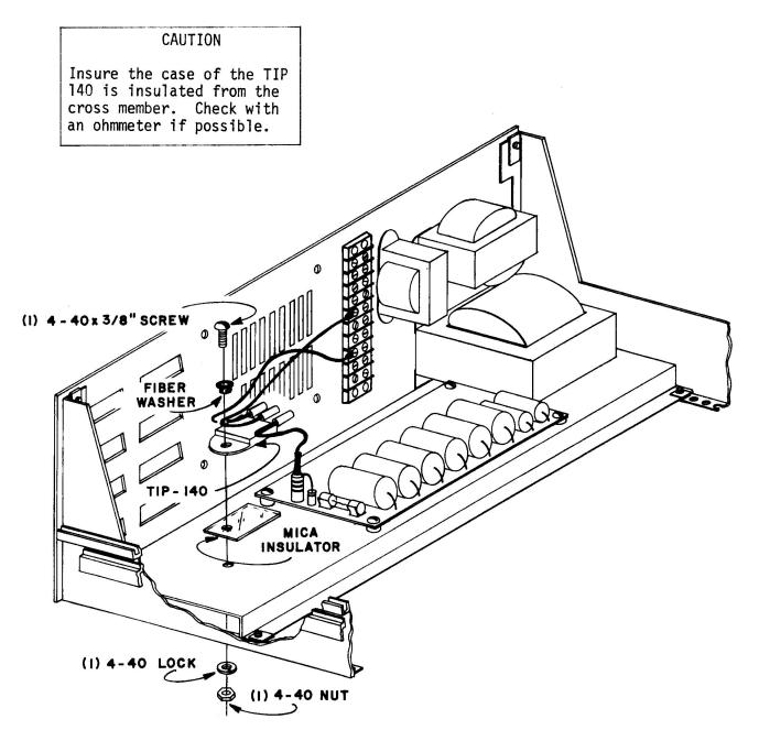
( ) Solder the 5 inch wire from B of the TIP 140 to the 47 ohm resistor and 9.1 volt zener connection. (See drawing)
