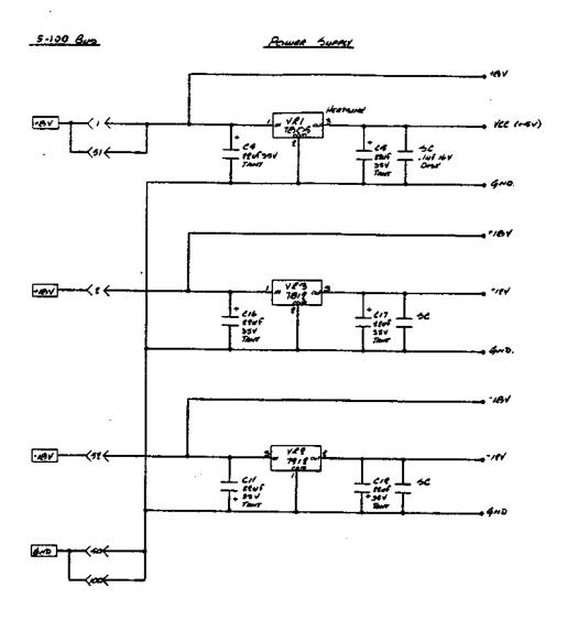
ATTACHE' SCHEMATIC DIAGRAMS 88-UIO BOARD (Sheet 4 of 4) VOLTAGE REGULATION
