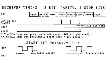
If the RSI line remains spacing for 1/2 a bit time, a genuine start bit is verified. Should the line return to a marking condition prior to 1/2 a bit time, the start bit verification process begins again.
