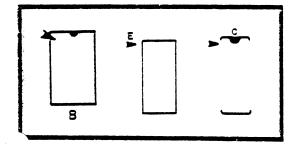
THE DRAWING ON THE LEFT INDICATES VARIOUS METHODS USED TO SHOW THE POSITION OF ICS ON THE PRINTED CIRCUIT BOARDS. THESE ARE SILK-SCREENED DIRECTLY ON THE BOARD. THE ARROWHEAD INDICATES THE POSITION FOR PIN 1 WHEN THE IC IS INSTALLED.
