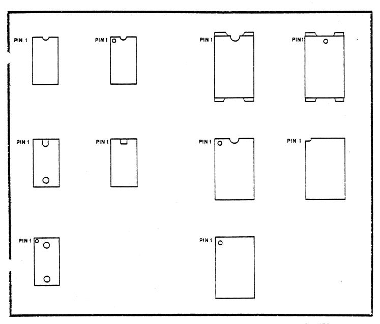
INTEGRATED CIRCUITS (ICs) CAN COME WITH ANY ONE OF, OR A COMBINATION OF, SEVERAL DIFFERENT MARKINGS. THESE MARKINGS ARE VERY IMPORTANT IN DETERMINING THE CORRECT ORIENTATION FOR THE ICs WHEN THEY ARE PLACED ON THE PRINTED CIRCUIT BOARDS. REFER TO THE ABOVE DRAWING TO LOCATE PIN 1 OF THE ICs, THEN USE THIS INFORMATION IN CONJUNCTION WITH THE INFORMATION BELOW TO PROPERLY ORIENT EACH IC FOR INSTALLATION.
