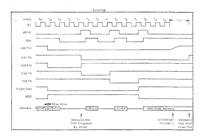
When U29 p9>1,  $\overline{SS}>1$ ,  $\overline{XRDY}>0$ , and the U15 data driver will be disabled. U29 p5>0, however, will force  $\overline{SS}>0$ ,  $\overline{XRDY}>1$ , and enable the U1 data driver, placing S8 - S15 on the bidirectional data bus. Since  $\overline{XRDY}$  is still high the processor will remain running.
