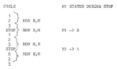
The processor is stopped for approximately 1 msec between each three cycle sequence. The oscilloscope will trigger at the start of each sequence and two different waveforms will be superimposed on the display.
