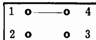
Cut etch jumper to change CPU clock
