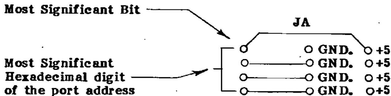
If it is necessary to change the port address for the board, cuts and jumpers in the JA block will be required.
