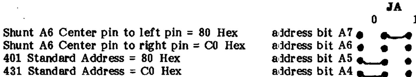
If it is necessary to change the port address for the board, cuts and jumpers in the JA block will be required.
