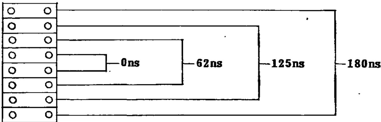
The standard selection is 125 nanoseconds for operation with Shugart or Remex Floppy Disk Drives.
