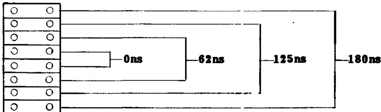
The standard selection is 125 nanoseconds for operation with Shugart floppy disk drives and 180 nanoseconds for Qume drives.
