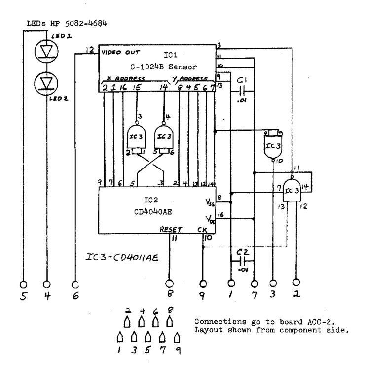
Schematic diagram of board ACC-1.
