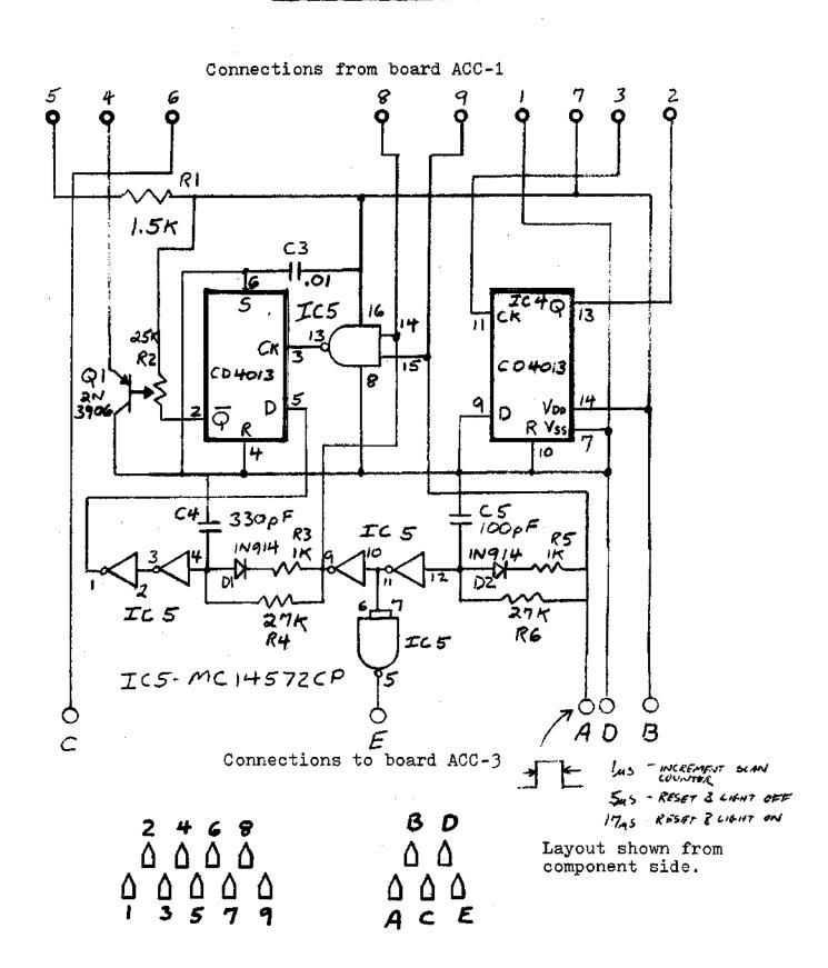
Schematic diagram of board ACC-2
