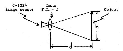
The relationship between the height of the object, h, the distance from lens to object, d, and the focal length of the lens, f, is given by this equation:
