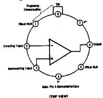
The leads of these ICs should be shaped into two rows of four and inserted in the IC socket in this order:
