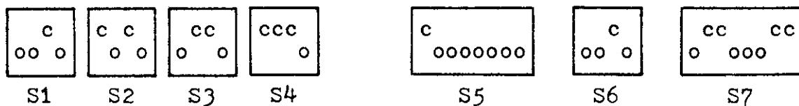
The next diagram (below) shows switch settings for a typical Cromemco system. The port address must be hex 40. Let byte bits 0 or 6 activate the bank and bit 0 be active on startup. Let the memory location be 16k to 32k.
