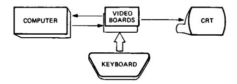
A universal asynchronous receiver transmitter (UART) performs the serial-parallel task between keyboard and computer; and computer and video memory. The video memory refreshes the screen. Timing and control logic addresses the memory and creates synchronization signals (syncs). The characters of the memory are mixed with the sync signals and are made available to the CRT chassis through a coaxial cable.
