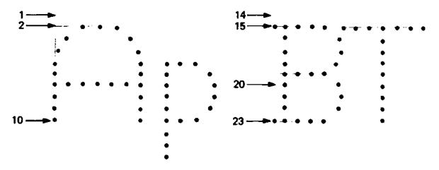
The data frequency is switching the beam on and off. The blank row between the p and t is produced by the generator itself. Vertical blanks between the characters is loading time for the shift register which follows the character generator. Each row is constructed of strata. All of this information in the Composite wave passes through a coaxial cable.
