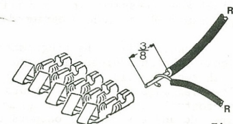
Figure 2 Knotted Red Wires
