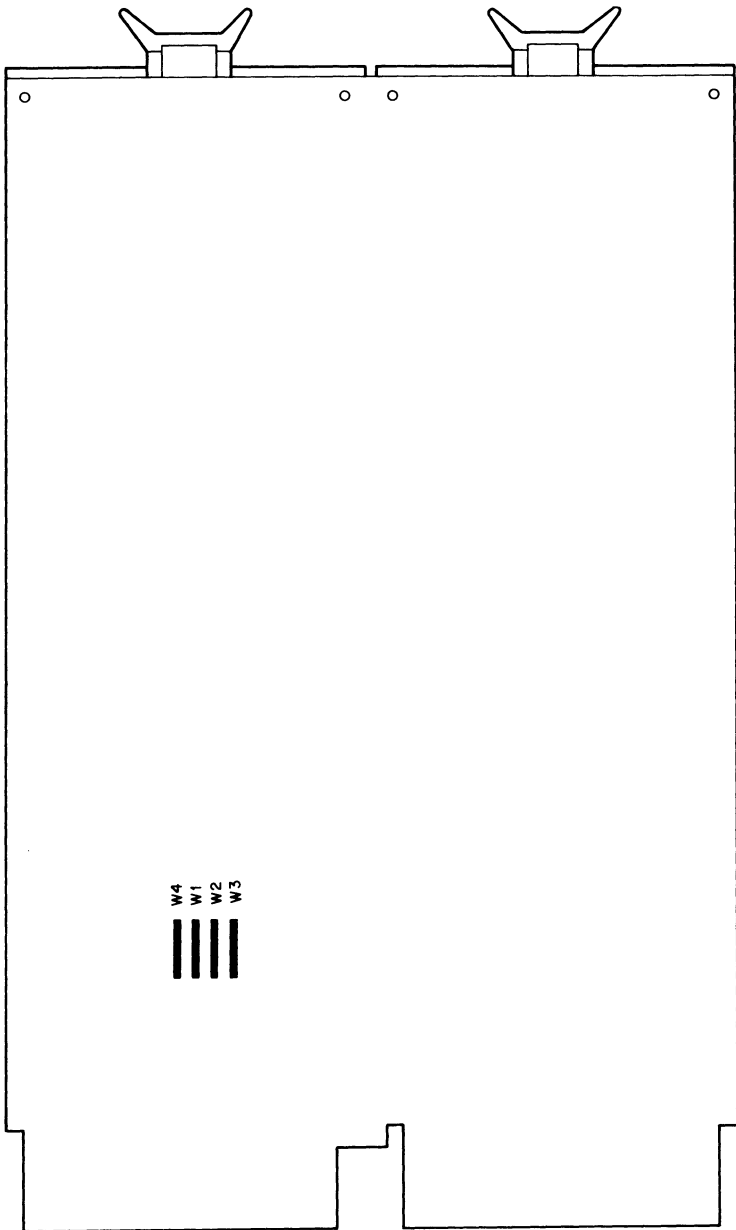
Figure 19-1 MSV11-B Jumper Locations
