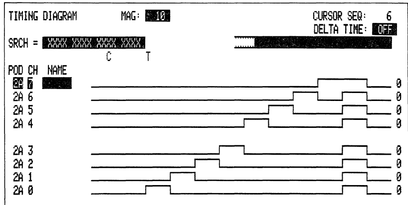
Figure 5-15. 5 μs pattern generator data acquired at 1 μs.
