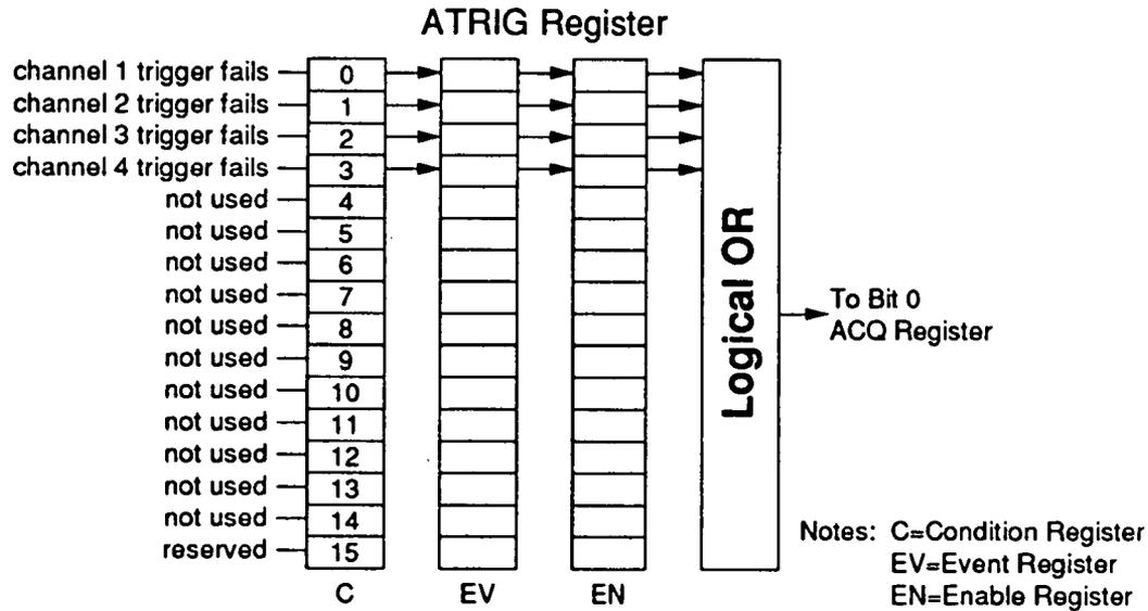
**Example      Query acquisition analog trigger event register**
