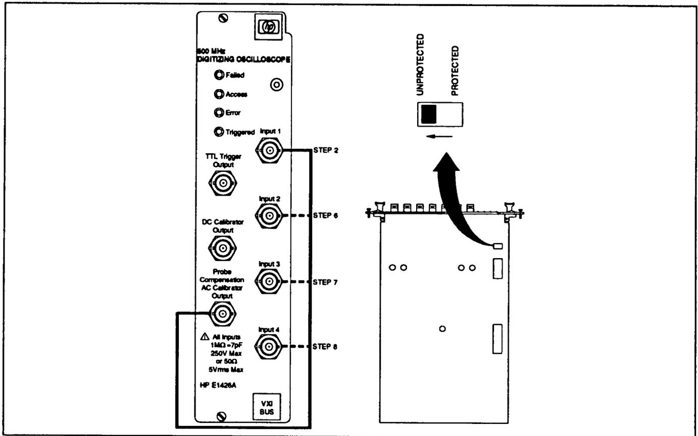
Figure 3-2. Example: Delay Calibration Setup
