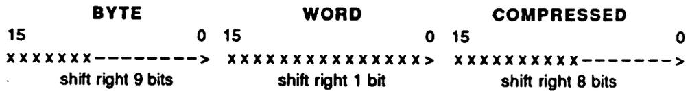
\*NOTE: x = bits to shift. The external buffers only contain the acquired waveform data, not preamble information. Preamble information can be read using the WAVEform:PREamble? query.
