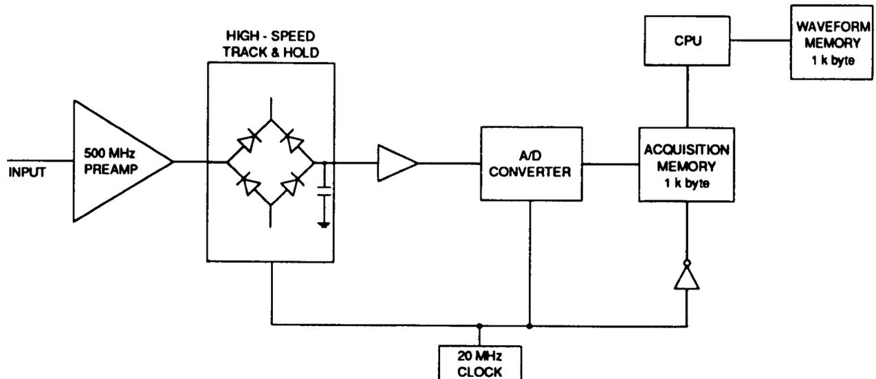
The preamplifier amplifies or attenuates (depending upon the sensitivity setting) the input signal to provide the Track and Hold circuit with the proper voltage range.
