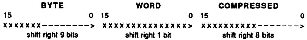
\*NOTE: x = bits to shift. The external buffers only contain the acquired waveform data, not preamble information. Preamble information can be read using the TRACe:PREamble? query.
