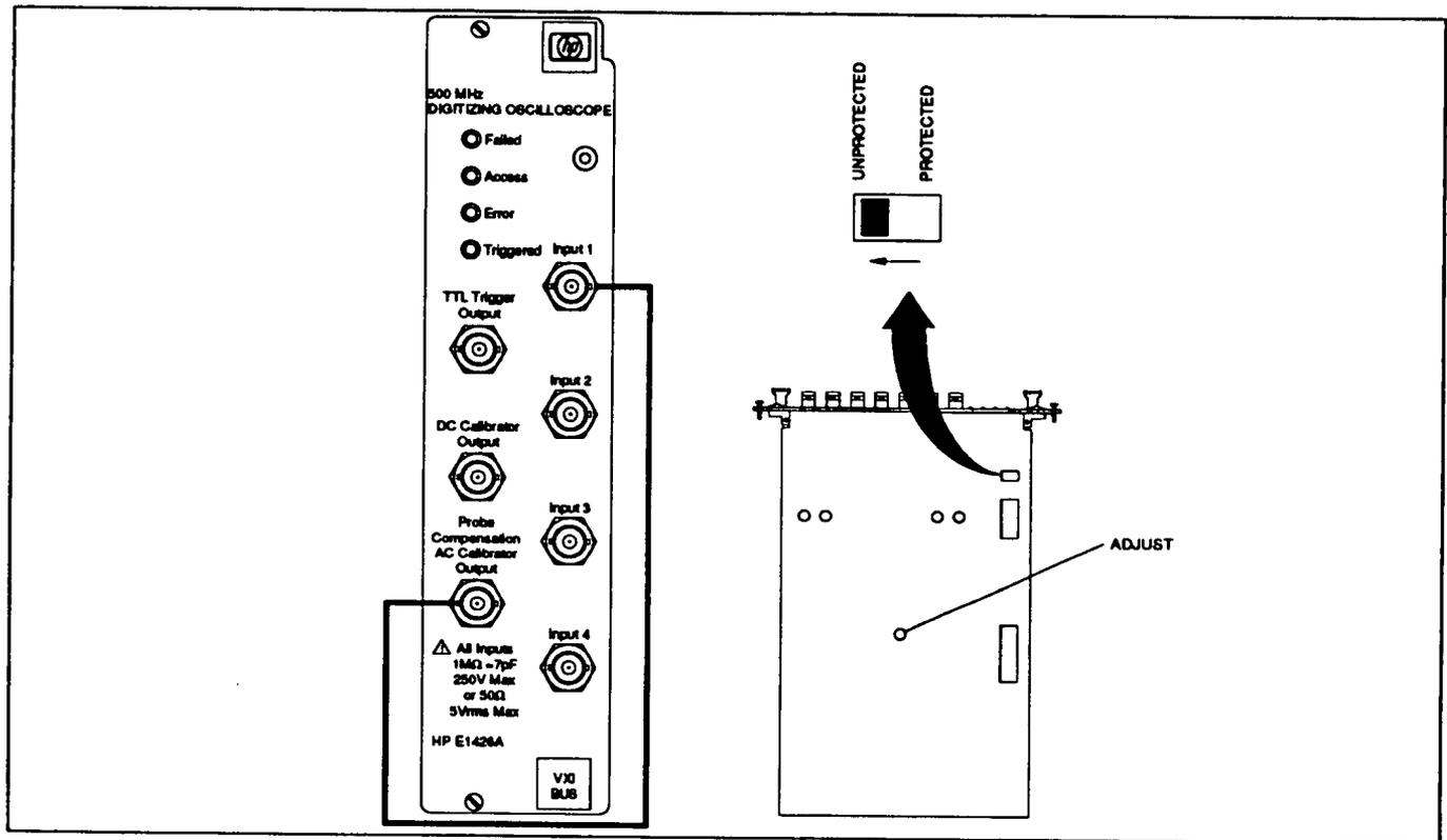
Figure 5-4. Example: Logic Trigger Calibration Setup
