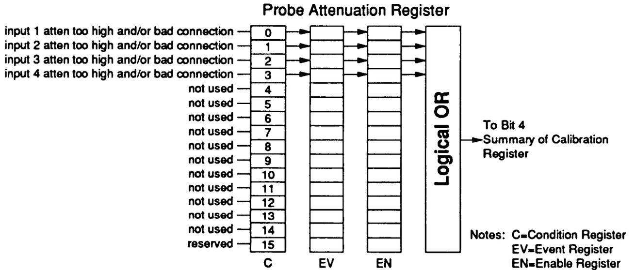
**Example Query probe calibration attenuation event register**
