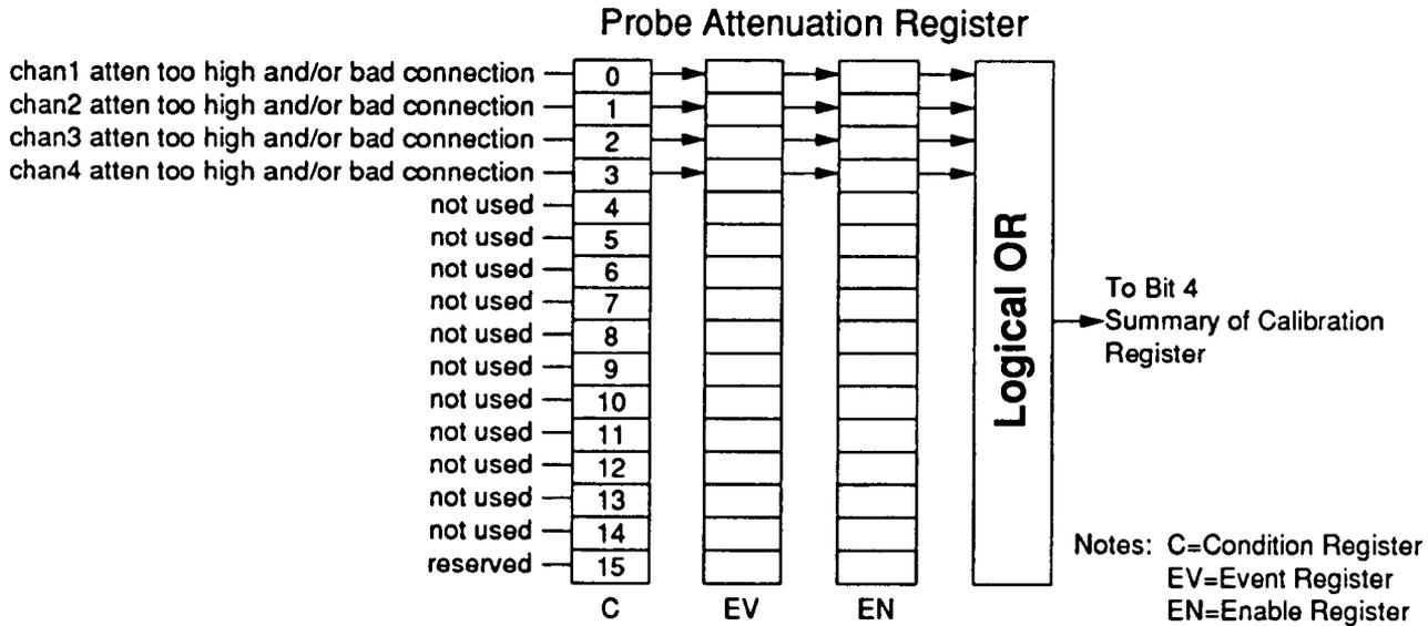
**Example    Query probe calibration attenuation event register**
