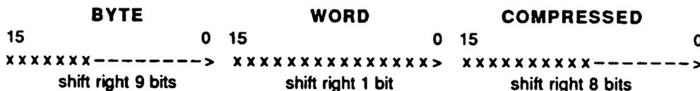
\*NOTE: x = bits to shift. The external buffers only contain the acquired waveform data, not preamble information. Preamble information can be read using the WAVEform:PREamble? query.
