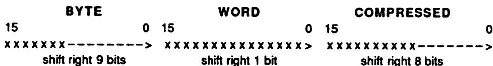
\*NOTE: x = bits to shift. The external buffers only contain the acquired waveform data, not preamble information. Preamble information can be read using the TRACe:PREAmble? query.
