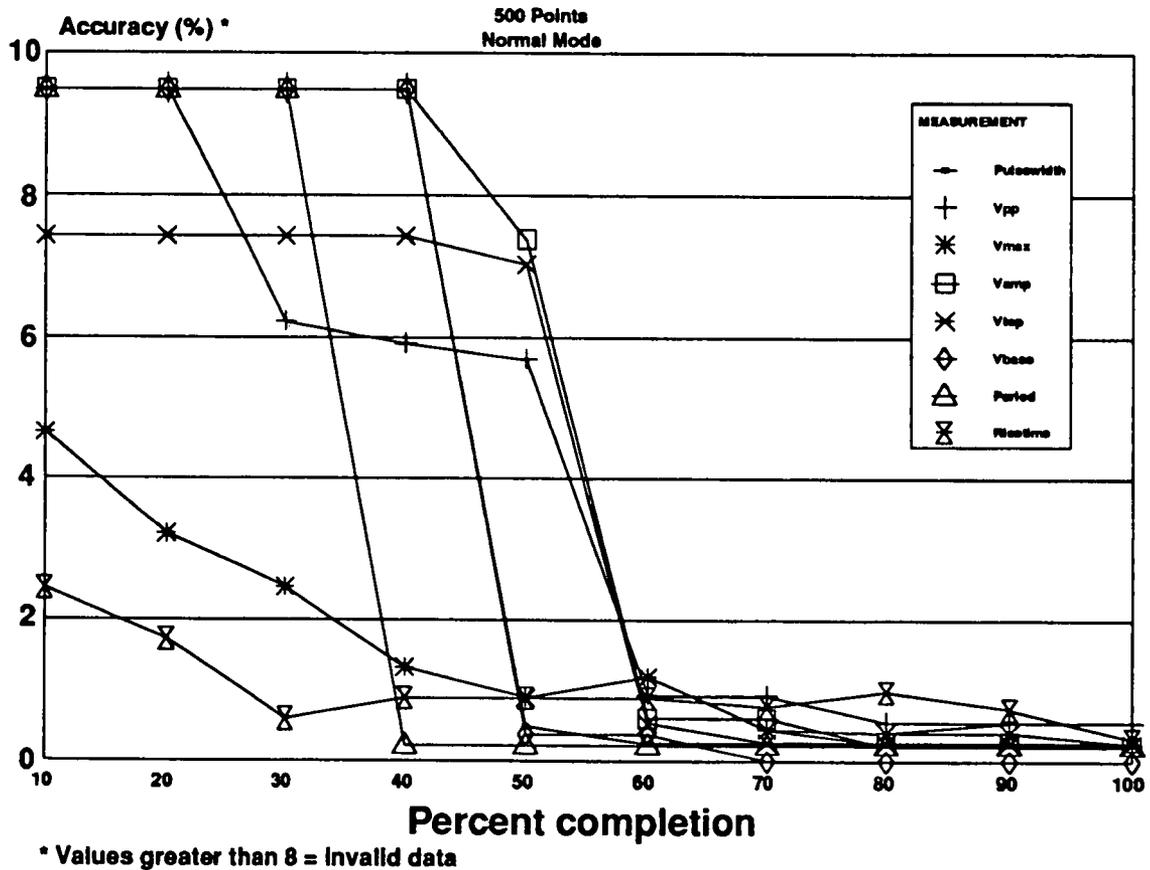
Note that any value over 8 actually represents invalid measurements because of lack of data points. From this data it can be seen that a completion criteria of greater than 60% does not improve the measurement accuracy very much. Some measurements, such as rise time, require even fewer points to provide accurate results.
