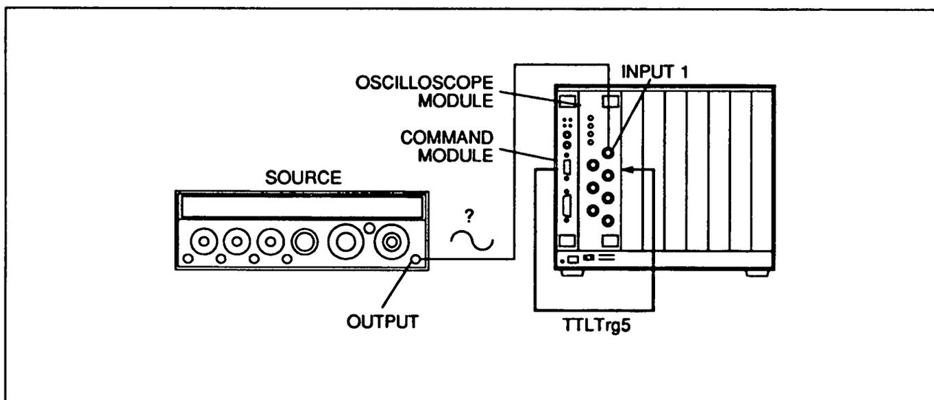
Figure 5-10. Example: Using the Backplane TTL Trigger
