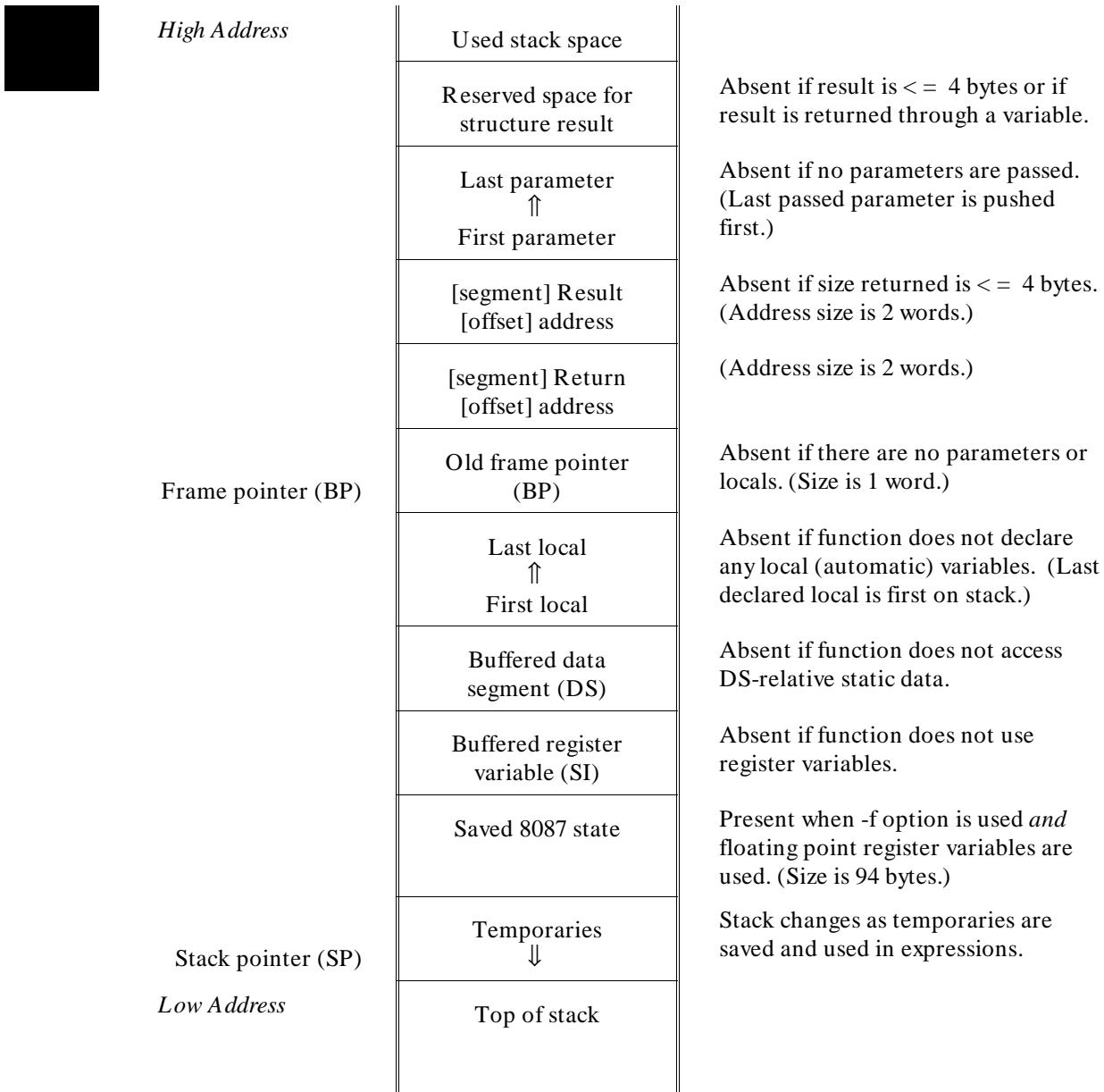
Figure 15-3. Stack for Large Memory Model
