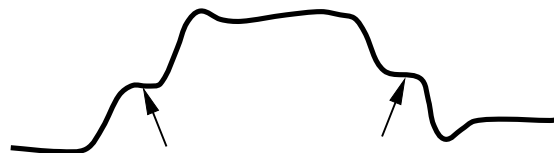
50% voltage "shelf" due to reflections.
