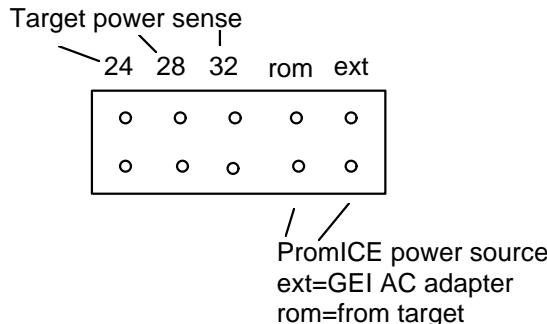
Set one jumper on either the "ext" pins for external power (preferred) or the "rom" pins for parasitic power (When using parasitic power, PromICE takes its power directly from the target's ROM socket. No external power supply should be connected to PromICE).
