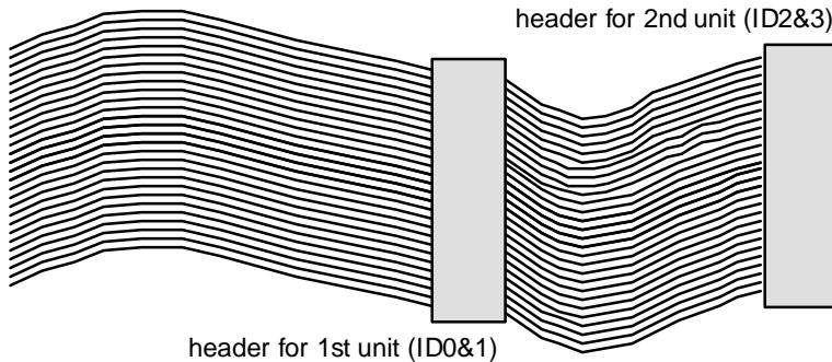
Connect the serial daisy chain adapter(s) as described in the previous section (1.3.2.3 *Multiple PromICEs on the serial link*). Connect the parallel bus cable in whatever way is most convenient.
