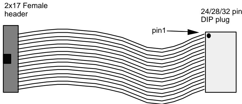
**WARNING:** CONNECTING THE CABLE INTO THE ROM SOCKET BACKWARDS WILL DAMAGE PromICE.
