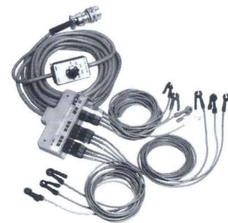
Ten-Lead Patient Cable Kit with V_1 through V_6 selector. Includes 10-ft. low-noise patient cable; 10 color-coded shielded lead wires with snap adapters, and a sample of disposable electrodes. 369500-28010
