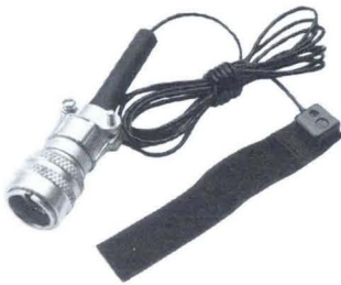
New infra-red, photoelectric plethysmograph records changes in pulsatile blood flow from fingers, toes, ear, forehead, etc. Miniature transducer attaches with velcro strap (supplied) or electrode type adhesive collars. Matched optics together with a unique two-stage IR-filter reduce the effects of ambient light and patient motion. 369500-31519
