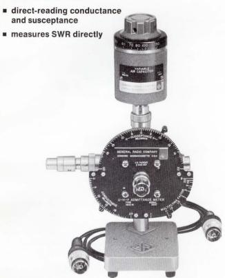
Versatile building block This null-type instrument measures complex impedance and admittance in coaxial systems and, as a reflectometer, will determine SWR, impedance magnitude, and reflection coefficient magnitude. It can be used to adjust a network to a predetermined admittance, to match one network to another, and to match antennas and other networks to 50-ohm circuits.
