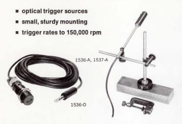
**Excellent trigger source** These photoelectric pickoffs produce an output whenever the photosensitive element senses a change in light such as that produced by a piece of reflective type on a moving object. The resultant pulses can be used to trigger a stroboscope so the flashes occur in synchronism with the motion, to permit the object to be viewed or photographed as though stationary. They can also be used to trigger oscilloscopes or electronic counters.
