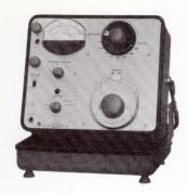
**Filter Characteristics:** BANDWIDTH between 3-dB points on selectivity curve: 1% of selected frequency. ATTENUATION, at 20% above and at 20% below selected frequency: > 50 dB referred to the level at the selected frequency. Attenuation at twice and at one-half the selected frequency is > 75 dB referred to the level at the selected frequency. Ultimate attenuation is > 85 dB. UNIFORMITY of filter peak response with tuning:  $\pm 1$  dB from 20 Hz to 6.3 kHz and  $\pm 2$  dB from 20 Hz to 20 kHz.
