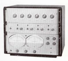
1654-Z1 Sorting System includes limit comparator for additional limits.
