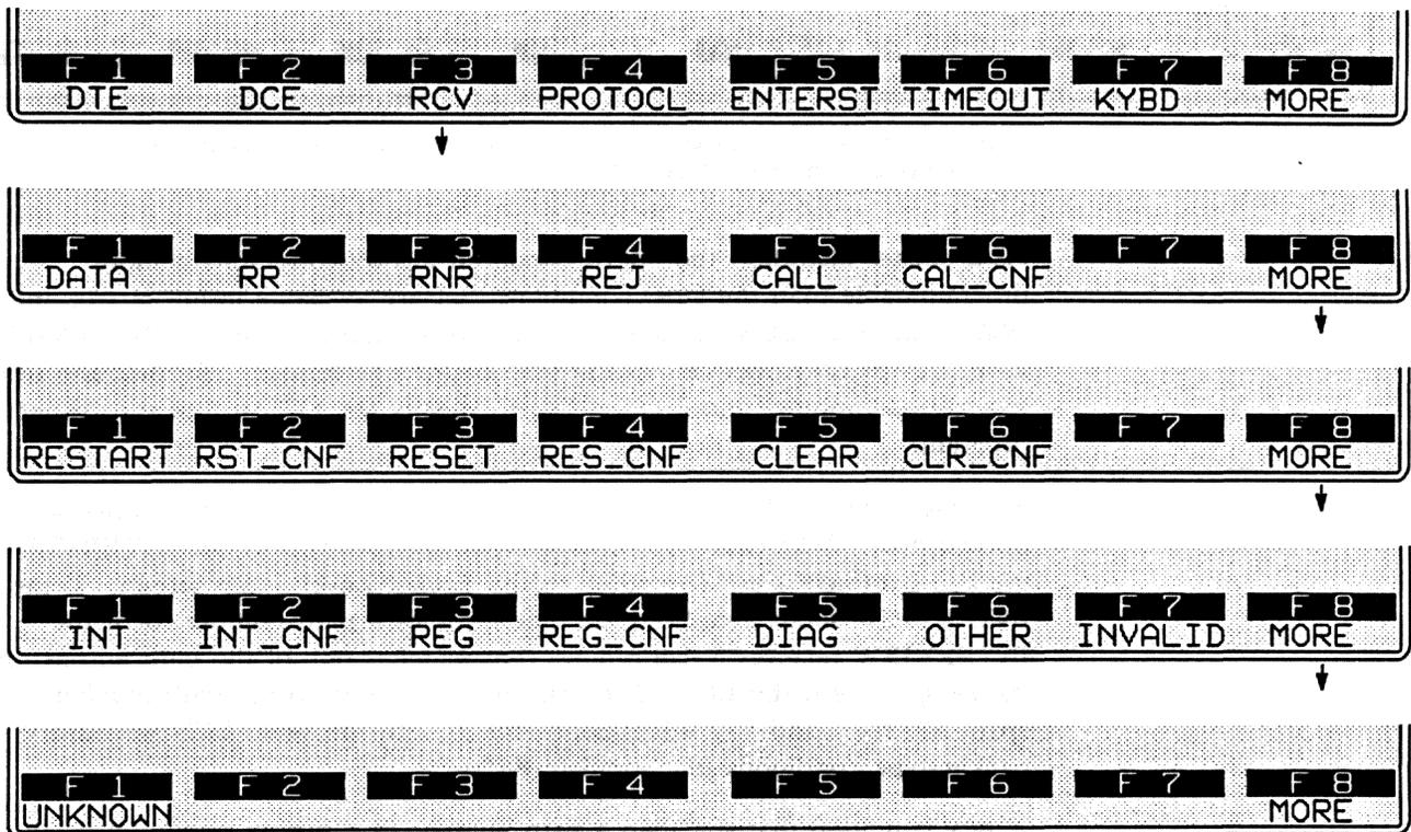
Figure 34-18 *INVALID* and *UNKNOWN* appear on the bottom two racks of RCV packet-type softkeys.
