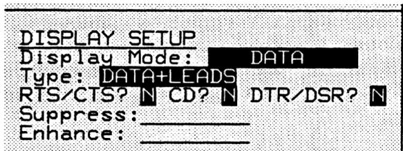
Figure 5-11 Five control leads are selectable under *Type: DATA+LEADS*.
