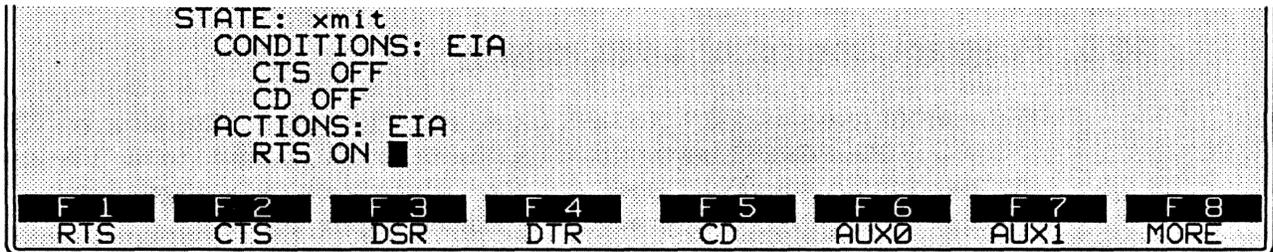
Figure 10-8 The spreadsheet program can control five RS-232 leads plus four auxiliary leads.
