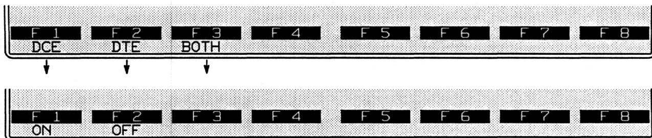
Figure 28-14 Screen display ("capture") can be turned on or off with respect to one data lead or both.
