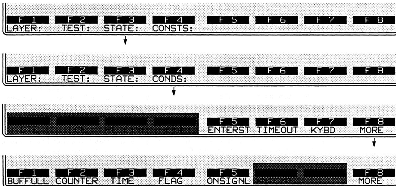
Figure 27-1 The eight layer-independent conditions are shown in the bottom two racks of softkeys.
