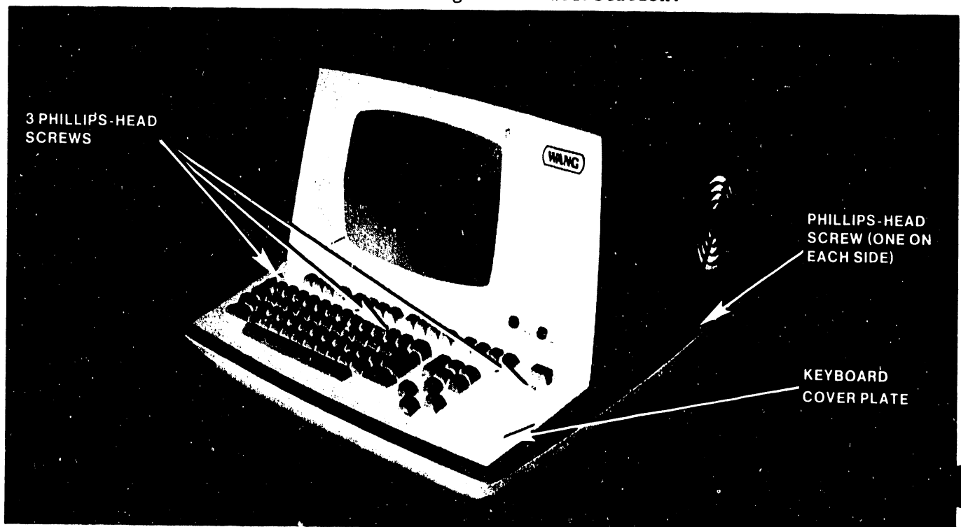
Figure 5-4. Cover Removal/Replacement
