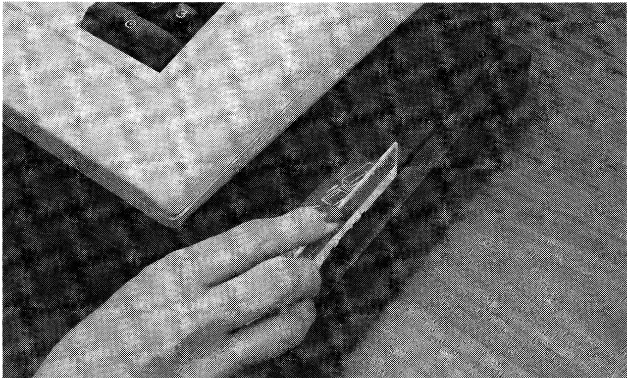
Figure 17. Magnetic Stripe Reader
