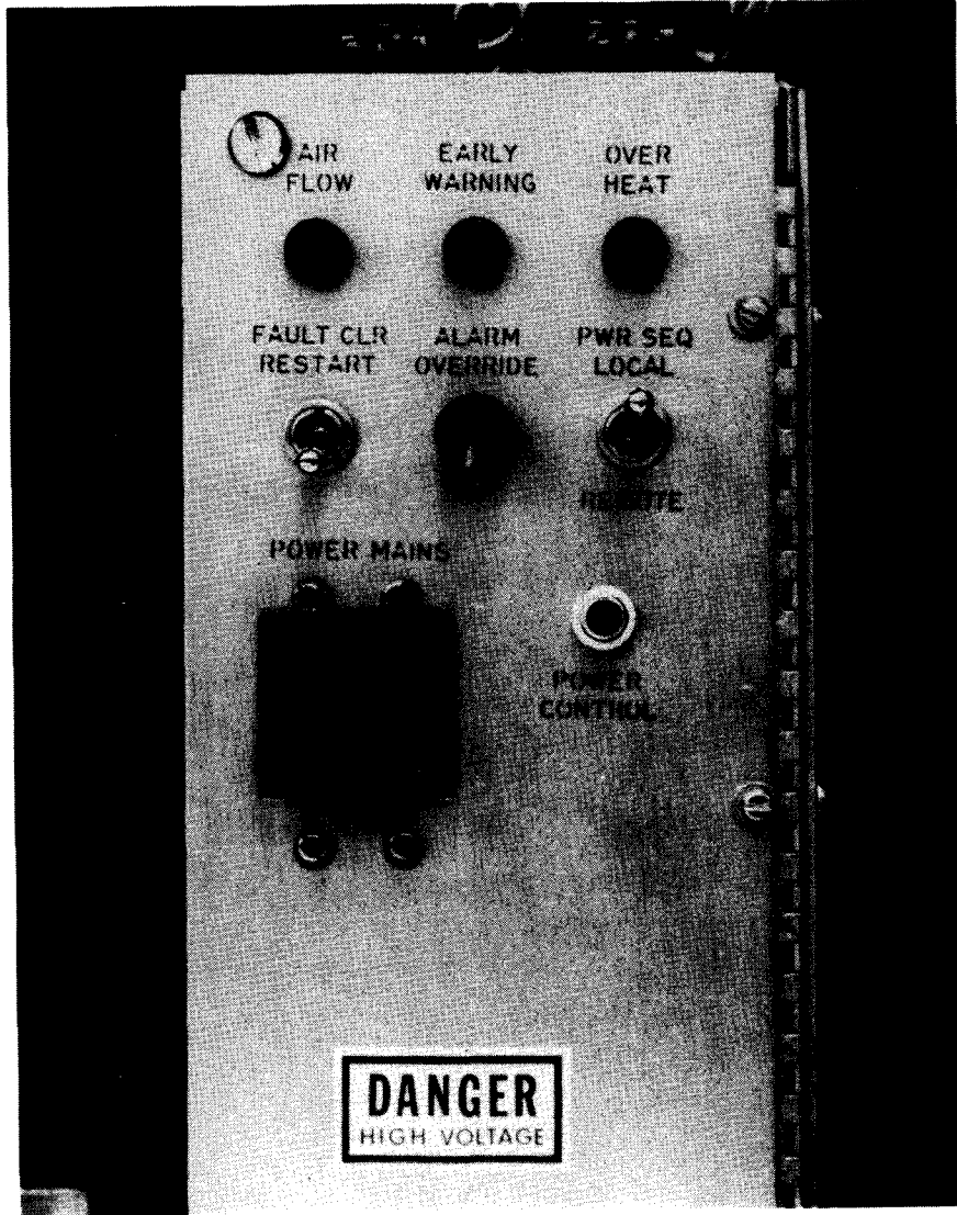
Figure 4-12. UNISERVO 10 or UNISERVO 14 Control Unit, Power Control Panel
