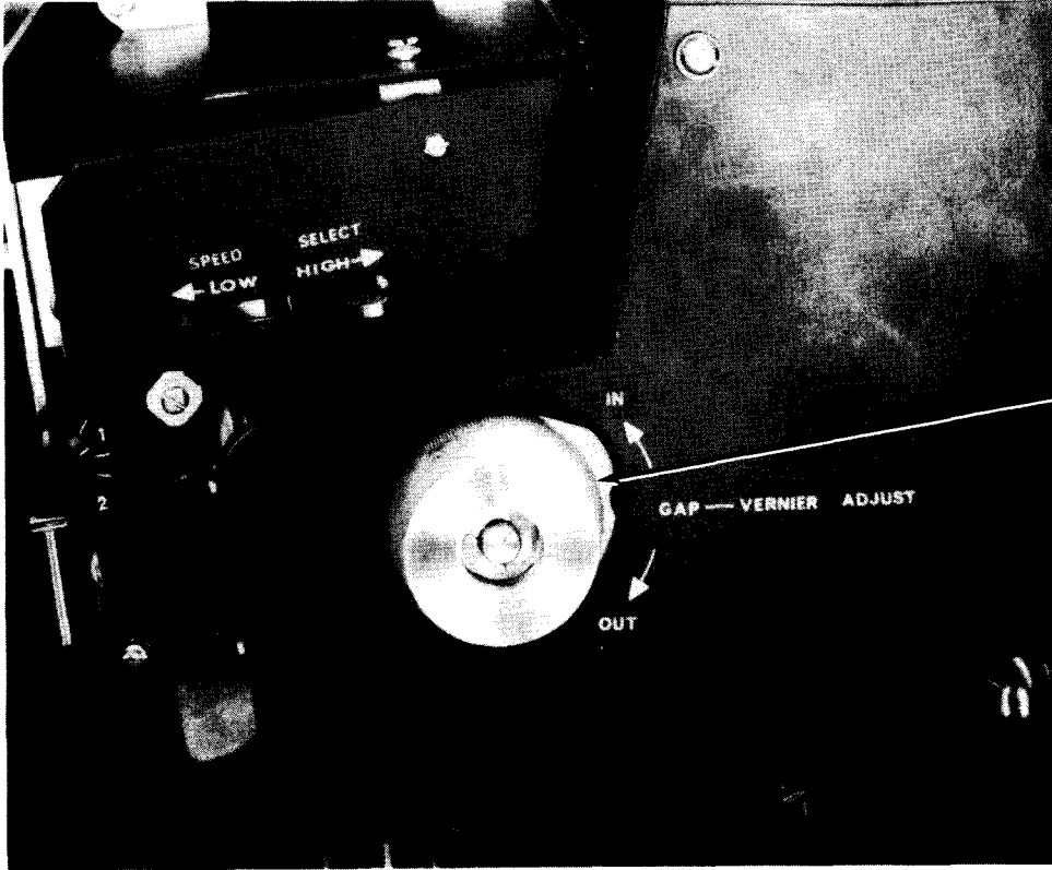
a. Print carriage open to show print gap manual vernier adjustment control
