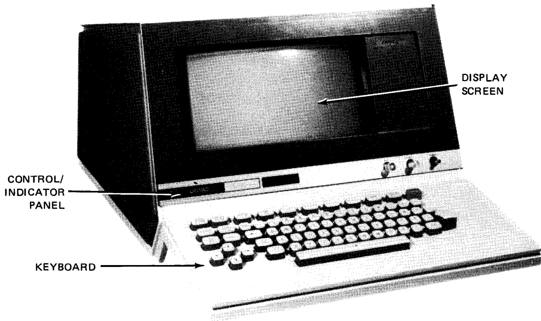
Figure 2—11. 90/30 or 90/30 B System, System Console ←
