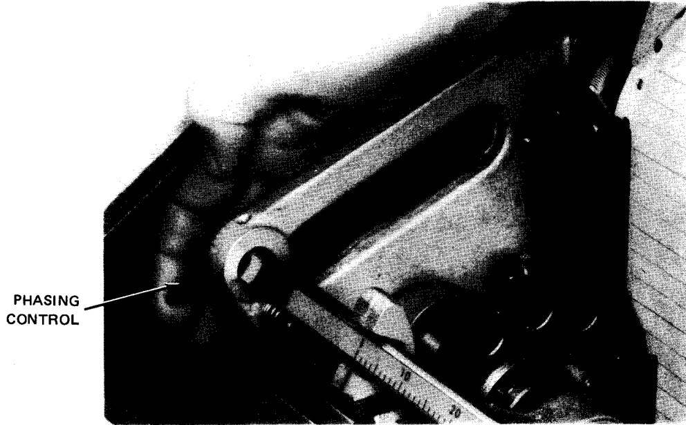
l. Adjusting phasing control to remove clipping
