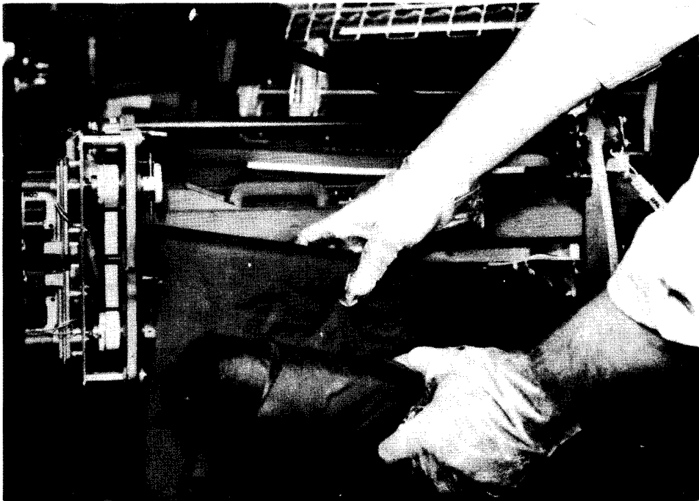
d. Removing upper and lower takeup spools
