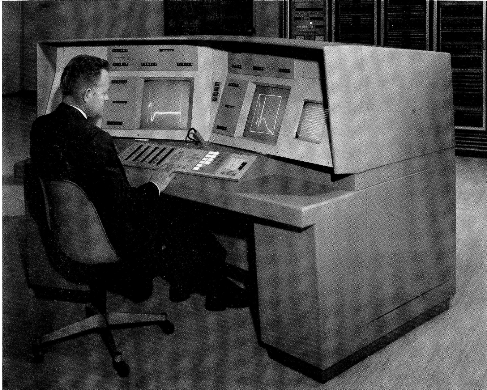
Figure 1. Control console used in the On-Line Computer Center.
