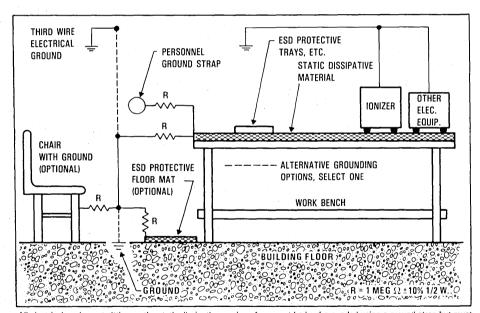
All electrical equipment sitting on the static dissipative work surface must be hard grounded using a ground strap but must be isolated from the static dissipative work surface.
