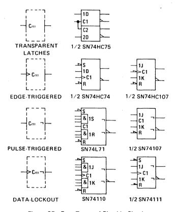
Figure 25. Four Types of Bistable Circuits
