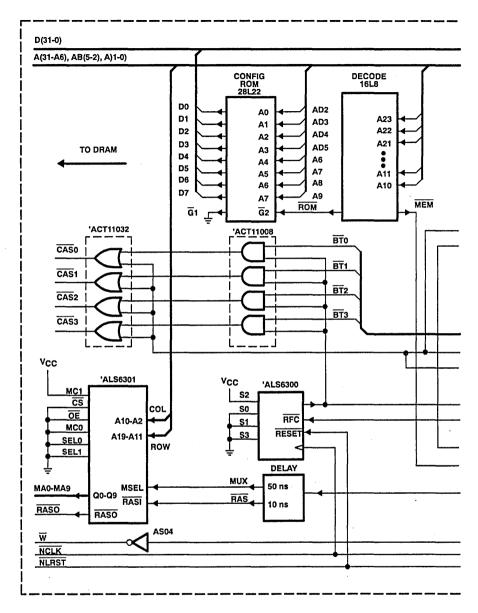
Figure 3. Typical NuBus™ Block Slave Application
