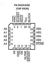
The 'ALS2442 is designed to support NuBus™ block slave transfers as defined by ANSI/IEEE Std 1196-1987. The 'ALS2442 interfaces directly with the 'ACT2440 NuBus™ controller and the 'BCT2420 NuBus™ transceivers. Figure 6 shows a typical NuBus™ interface when using the 'ALS2442 with the 'ACT2440 and 'BCT2420.
