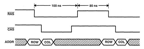
Figure 1. Typical DRAM Access Cycle Timing
