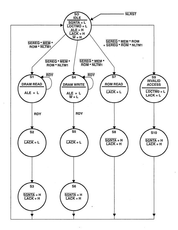
Figure 2. State Diagram for NuBus™/Memory Controller ('82S167)
