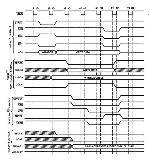
Figure 5. Normal (Nonblock) Write Cycle
