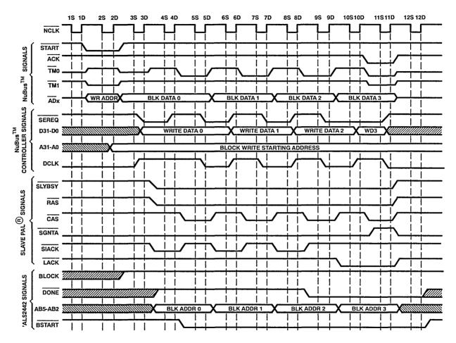
Figure 7. Block Write Transfer (4 Words)
