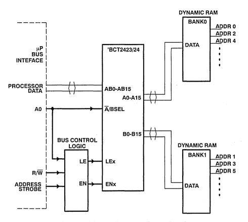
Figure 3. Memory Interleave System Interface
