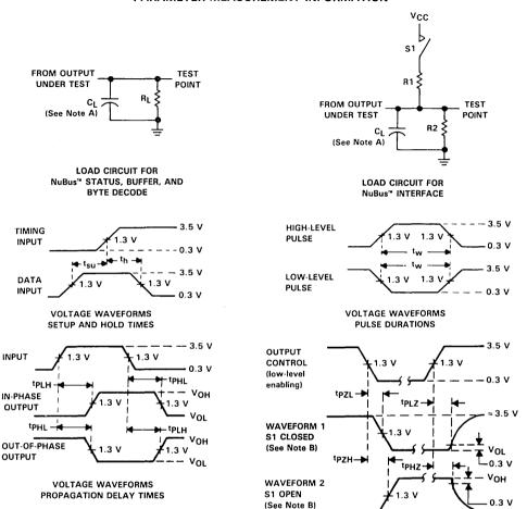
VOLTAGE WAVEFORMS ENABLE AND DISABLE TIMES, THREE-STATE OUTPUTS
