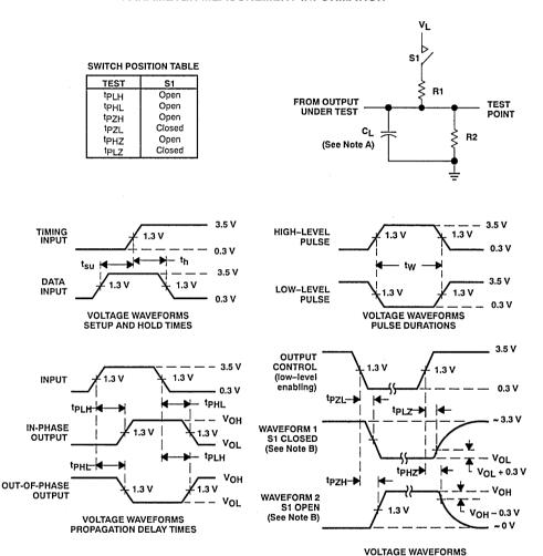
NOTES: A.C. includes probe and jig capacitance.
