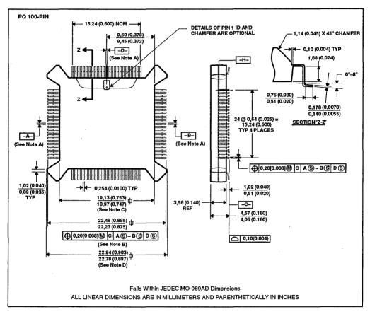
NOTES: A.Datums A-B and -D- to be determined where center leads exit plastic body at plane -H-.
