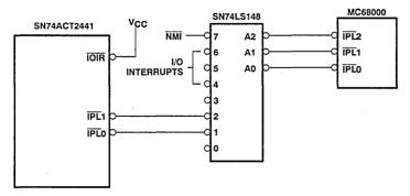
Figure 3. Expanding Interrupts to the MC6800
