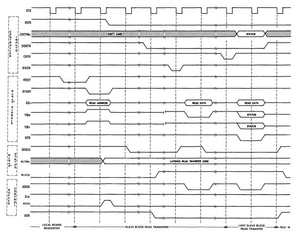
$<sup>^{\</sup>dagger}$ The BLOCK signal must be supplied by external logic, such as from Tl's SN74ALS2442.
