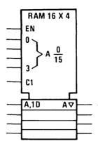
Figure 24. Array of 16 Sections of Four Transparent Latches with State Outputs Comprising a 16-Word × 4-Bit Random-Access Memory
