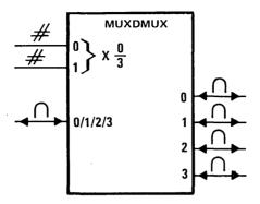
Figure 14. Analog Data Selector (Multiplexer/Demultiplexer)
