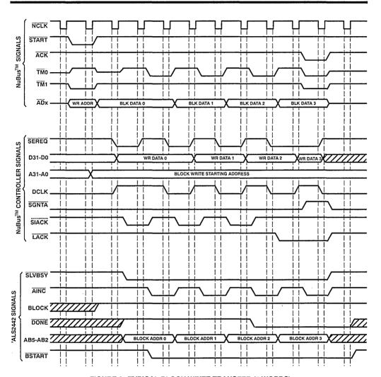
FIGURE 2. TYPICAL BLOCK WRITE TRANSFER (4 WORDS)
