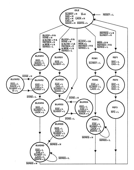
Figure 10. Slave PAL® State Diagram
