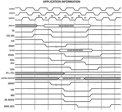
† The timing diagram assumes the asynchronous inputs FC1-FC0, BG, XBR, XBACK, and IOIR are recognized at the next falling CLK edge.
