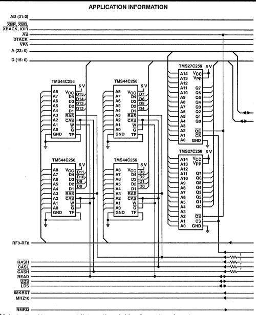
† Series damping resistors are recommended but may not be required depending on system environment.
