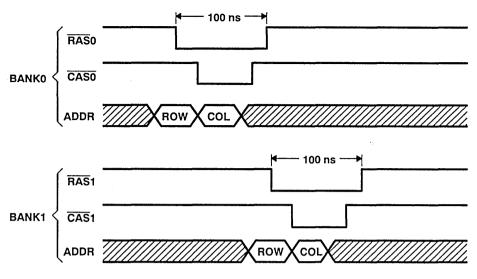
Figure 2. Two-Way DRAM Access Cycle Timing
