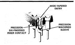
Inner contact - 30  $\mu$ in gold over 50  $\mu$ in nickel or 100  $\mu$ in tin/lead over 50  $\mu$ in nickel
