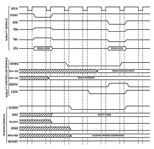
FIGURE 3. TYPICAL NONBLOCK READ TRANSFER CYCLE
