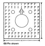
NOTE: Socket electrical pin-out pattern represents component side of P.C.B. layout. (TYP. counter clockwise numbering pinout system.)
