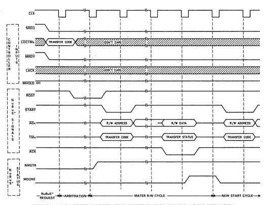
FIGURE 4. HIGH-SPEED MASTER READ/WRITE CYCLES (MHOLD LOGIC NOT USED)
