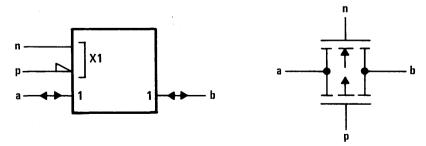
Figure 13. CMOS Transmission Gate Symbol and Schematic
