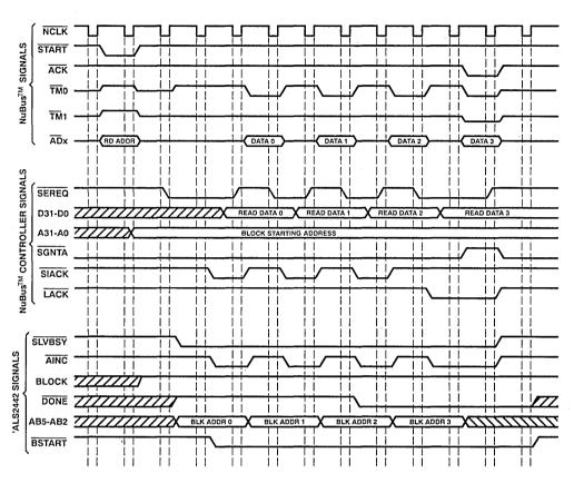
FIGURE 1. TYPICAL BLOCK READ TRANSFER (4 WORDS)
