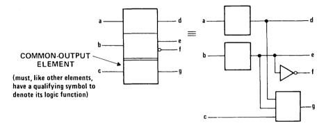
Figure 3. Common-Output Element
