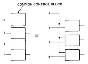
Figure 2. Common-Control Block
