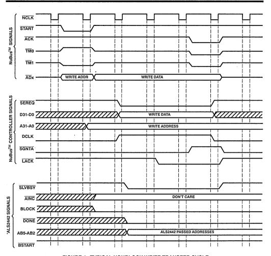
FIGURE 4. TYPICAL NONBLOCK WRITE TRANSFER CYCLE
