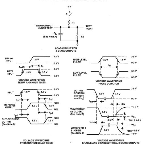
NOTES: A.C<sub>L</sub> includes probe and jig capacitance and is 50 pF for  $t_{pd}$  and  $t_{en}$ , 5 pF for  $t_{dis}$ .
