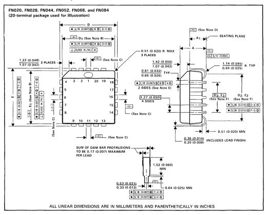
NOTES: A. All dimensions conform to JEDEC Specification MO-047AA/AF. Dimensions and tolerancing are per ANSI Y14.5M-1982.
