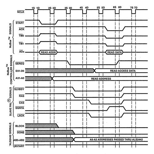
Figure 4. Normal (Nonblock) Read Cycle
