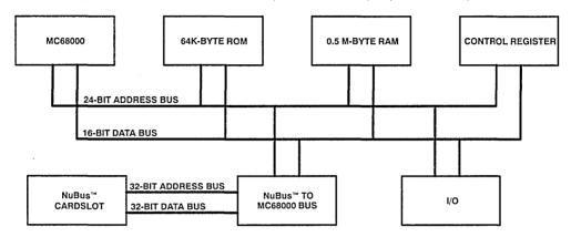
Figure 7. System Block Diagram Showing Data Paths
