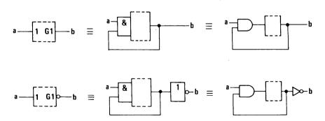
Figure 5. G Dependency Between Outputs and Inputs
