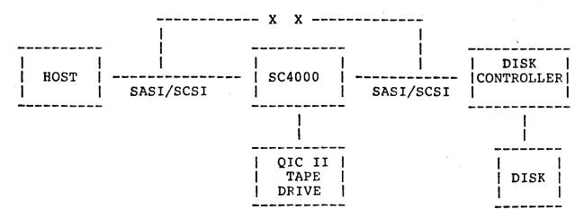
The broken path shown might have been the orginal system set up before installing SC4000 and QIC II tape drive.
