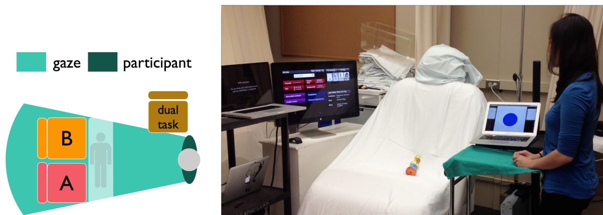
Figure 7: Overhead view of experimental setup with scenario [A] and displayed aid [B] (left). Participant uses dynamic aid while responding to questions (right), with color task visible and adjacent.
