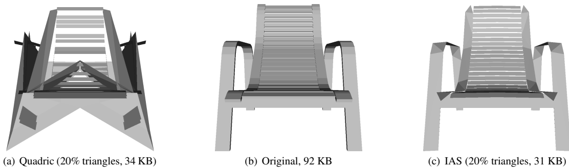
Figure 9: Patio chair with highly instanced slats from Table 3 simplified to 20% of the original triangle count. IAS results in surprisingly better quality than the reference implementation of quadric simplification.
