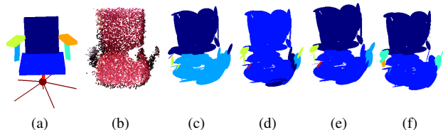
Figure 5: In the recognition phase, we use a MRF formulation to match the learned chair model (a) to the input scan (b). While simply matching height (c) or relative size (d) results in wrong matches, we correctly identify the chair back and seat (e) using both the terms. The most likely assignment adding binary term is shown in (f). Note in areas of very sparse data, there can still be mismatches, requiring further refinements, especially for small parts, e.g., we fail to extract symmetry between the chair arms in this example.
