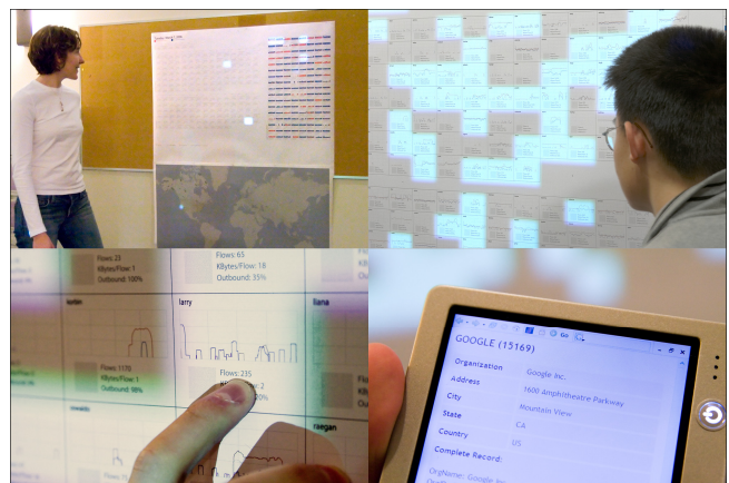
Figure 5. The network awareness GIGaprint provides multiple levels of interaction. From top-left to bottom-right: 1) It projects an ambient display showing the activity of different machines in the network. 2) In close reading , a user may inspect the printed information. Within arm’s reach, the user enters the interaction phase. The user may also inspect private information with his mobile
