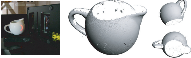
Figure 2: Left: Acquisition setup with Cyberware Desktop 3D Scanner 15 and physical model, right: Raw point cloud obtained from six range images in a single rotational scan. The spiky outliers are artifacts caused by specular reflections.
