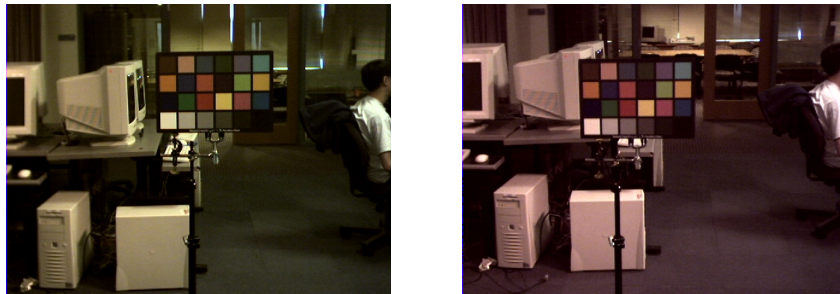
Figure 1: Color variations across image sensors. These two images were taken at the same time from adjacent cameras under typical lab light levels. The cameras are made with the same CMOS image sensor. The settings affecting color balance and color gain are identical, yet there is a significant perceptible color difference between these two images.
