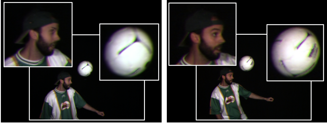
Figure 14: Spatiotemporal optical flow. Optical flow is an application that relies heavily on color calibration as it has a central assumption of brightness consistency. Perceptual color differences are still undesirable, but of greater concern are numerical differences. Four Images acquired from different locations and at different times are aligned with multi-dimensional optical flow. Left: Data acquired from a partially calibrated setup shows noticeable flow inaccuracies on the fine details such as the person's eye. The soccer ball is relatively sharp. Right: Data from a second acquisition after full calibration with full post-processing applied. The details of the eye are preserved and the soccer ball is sharper.
