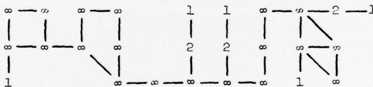
Figure 2. The l function for the example graph in Figure 1; there are three chains of length 2.
