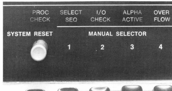
Figure 10. MANUAL SELECTOR Switches and Indicator Lights for ALPHA ACTIVE, OVER FLOW, SELECT SEQUENCE, I/O CHECK, and PROC CHECK Conditions.
