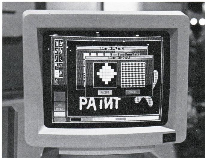
The Pattern Editor allows creation of customized backgrounds and overlays in eight mixed colors.
