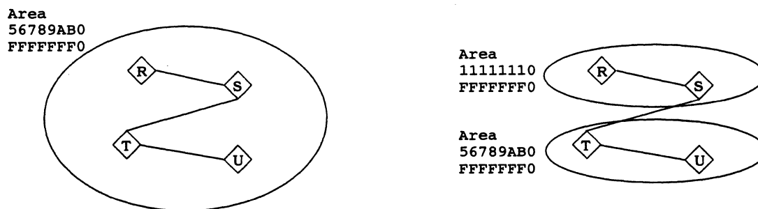
Figure 2-10: Splitting a Routing Area
