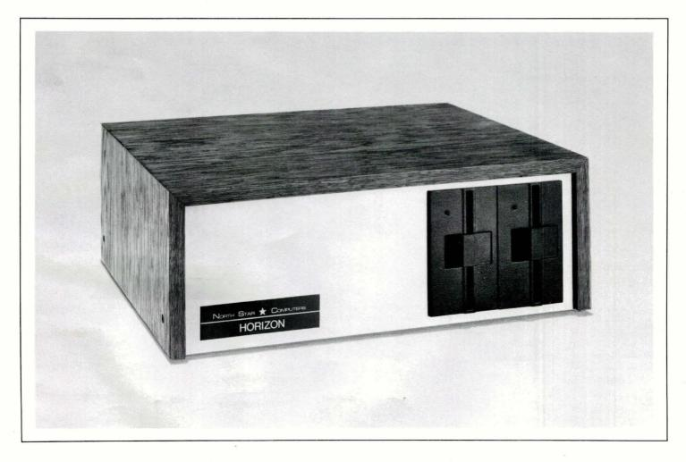
The **HORIZON** Computer is a complete, high-performance microcomputer system with integrated floppy disk memory. To begin programming in North Star extended disk BASIC, merely plug in a CRT or hard-copy terminal. Operating a HORIZON is simple: there is only an on/off switch and a restart button. The North Star software is loaded from diskette within seconds after power-on.
