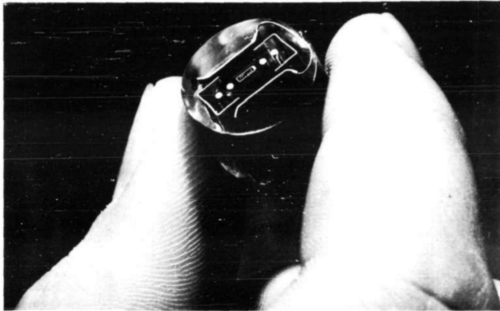
Fig. 3-2. Section of 6AN5 tube cast in clear resin for dimensional analysis.
