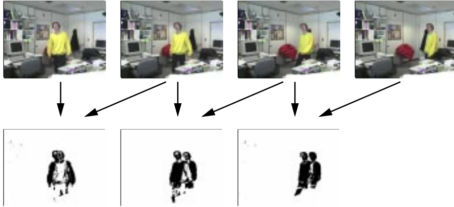
Figure 4-14: The output of VsDiffMotion with the shadow artifact
