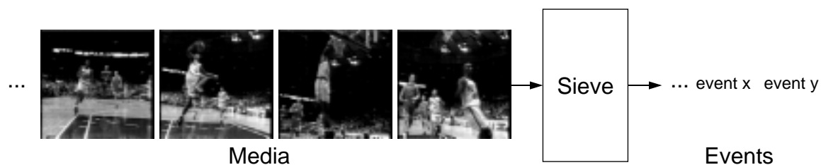
Figure 3-1: Transforming unstructured media into symbolic events
