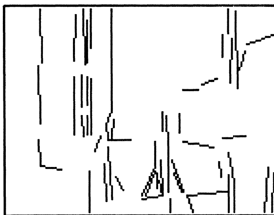
Figure 4-2: Matched stereo edges for the stereo pair in Figure 4-1. Each edge point is labeled with its 3-D coordinates.
