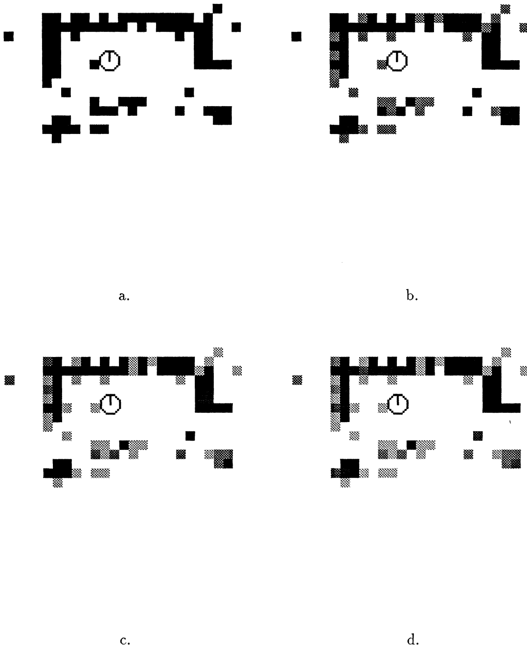
Figure G-7: Examples of the final Room 914 model using the linear update algorithm with Hysteresis = 4 and various rise times.
