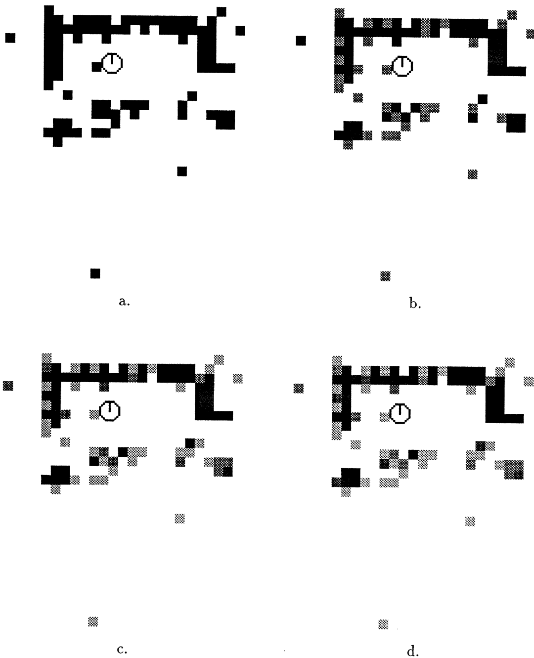
Figure G-9: Examples of the final Room 914 model using the linear update algorithm with Hysteresis = 5 and various rise times.
