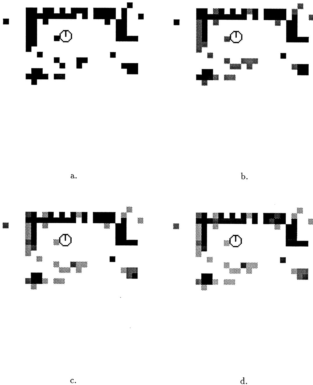
Figure G-5: Examples of the final Room 914 model using the linear update algorithm with Hysteresis = 3 and various rise times.
