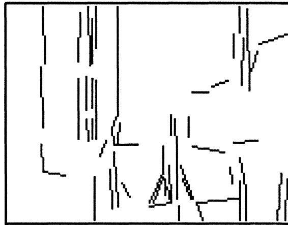
Figure 1-3: Matched stereo edges for the stereo pair in Figure 1-2. Each edge point is labeled with its 3-D coordinates by the stereo system.
