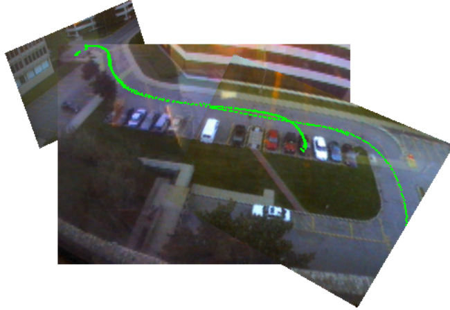
Figure 7: An example of an error. Two vehicles travelling close together (about two cars lengths apart) were assigned the same unique identifier.
