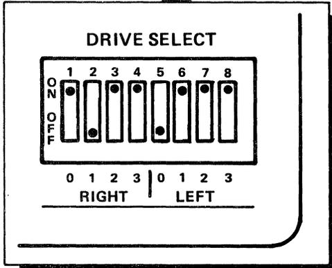
**NOTE:** Dots shown in the above figure indicate that switches 2 and 5 are set on (pushed in). The switches are factory set to this position and you need not reset them.
