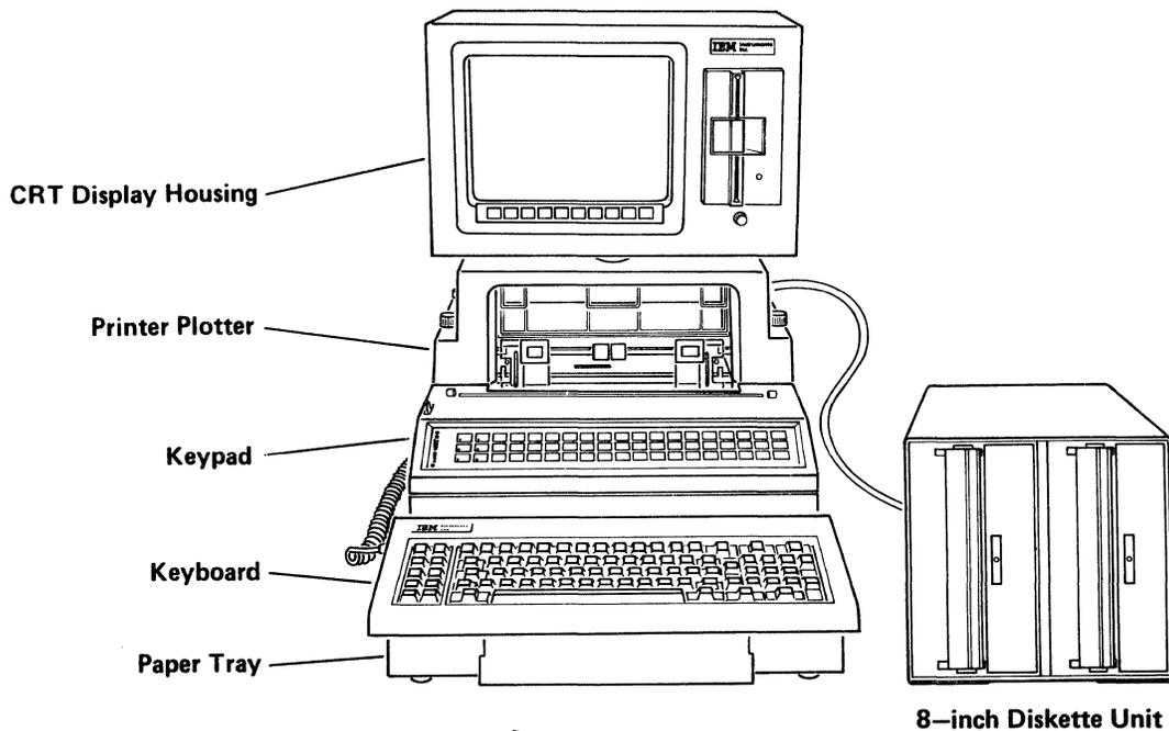
Figure 1-1. The IBM Instruments Computer System.
