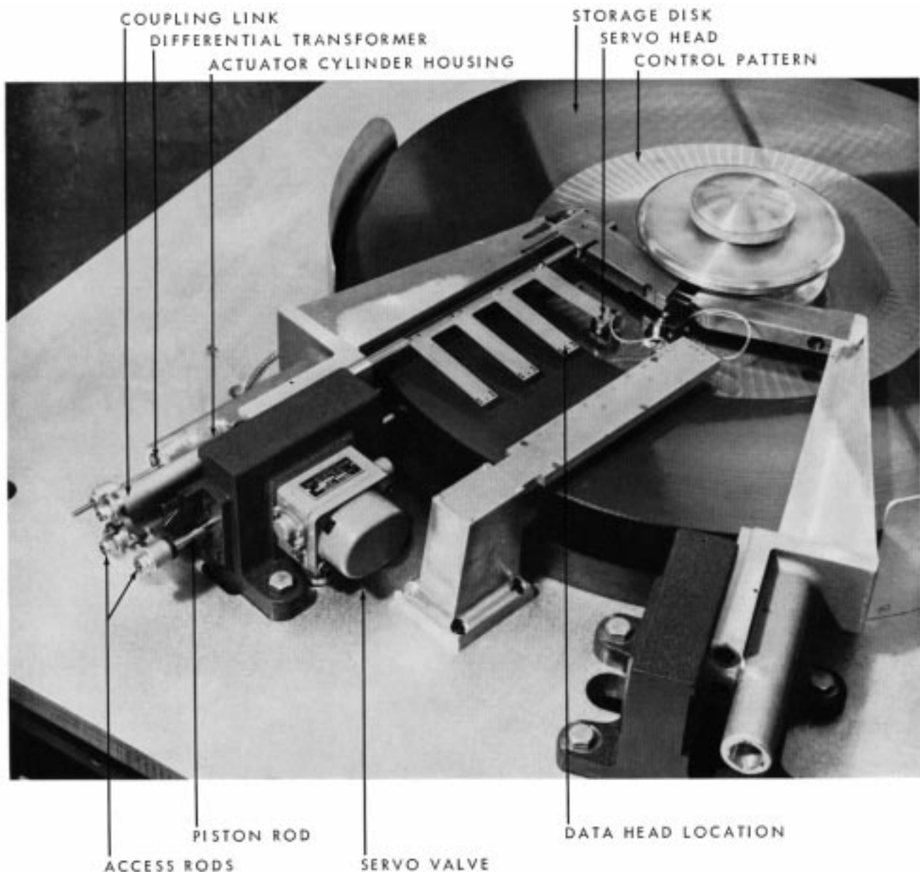
Figure 1 Servo-access mechanism.
