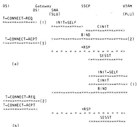
Figure 7 Sequence diagrams for establishing transport connection: (a) from the OSI side; (b) from the SNA side. See discussion in text.
