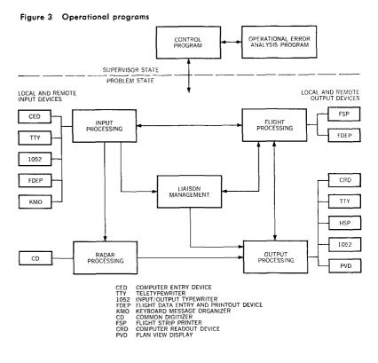
Teletype equipment at flight service stations, airline offices, and military operation offices may communicate with the 9020 system. High-speed circuits are used to pass data to and from adjacent computer-equipped centers, to and from flight-data entry and printing devices at airport control towers and Terminal Radar Approach Control Facilities (TRACON'S), and from the special devices that provide digital radar data from each radar site.
