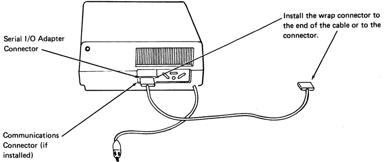
4. After you install the wrap connector, press the EXECUTE key. One of the following messages is displayed, giving you the results of the test:
