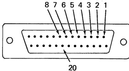
**Terminal Cable I/O Device Connector Socket**
